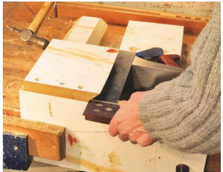
▲ Pic.8 Fitting the back of the mitre box. Make sure it is square; note the hammer. It is easier to locate a component by tapping gently than by pushing
